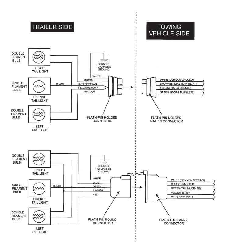
Figure 79. Trailer Wiring Diagram (5-Pin)
